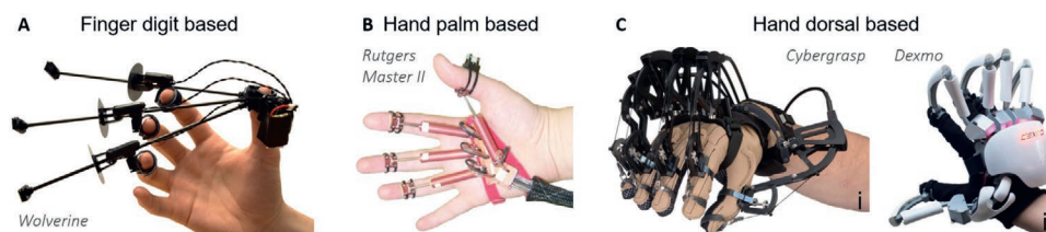
Figure 10. Different integration of hand kinesthetic haptic feedback devices A) between fingertips and thumb, [137] B) on hand palm [144] and C) on the back of the hand. [147,148] (A) reproduced with permission. [137] Copyright 2016, IEEE; (B) reproduced with permission. [144] Copyright 2002, IEEE; (C-i) reproduced with permission. [147] Copyright CyberGlove Systems; (C-ii) reproduced with permission. [148] Copyright 2020, Dexta Robotics.
